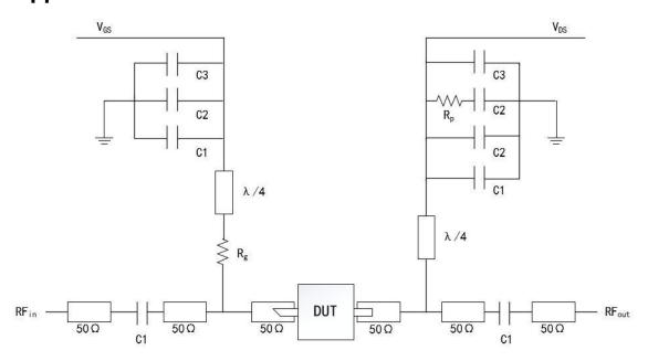
DUT: Device to be tested
