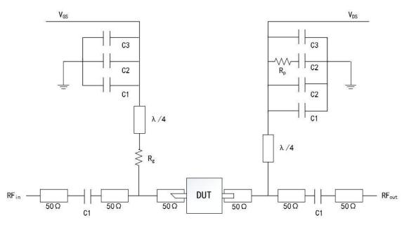
DUT: Device to be tested
