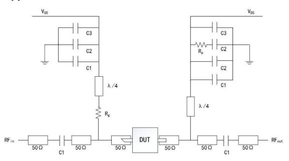
DUT: Device to be tested
