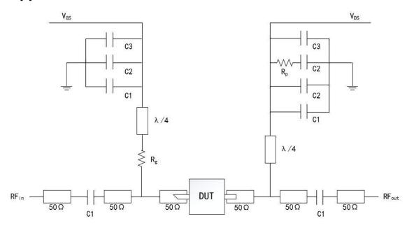
DUT: Device to be tested
