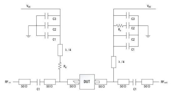
DUT: Device to be tested
