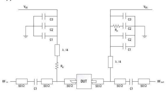
DUT: Device to be tested
