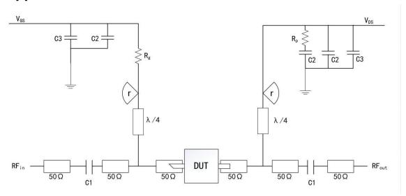
DUT: Device to be tested
