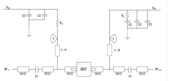
DUT: Device to be tested
