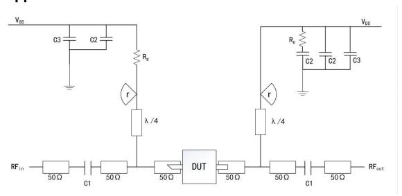
DUT: Device to be tested
