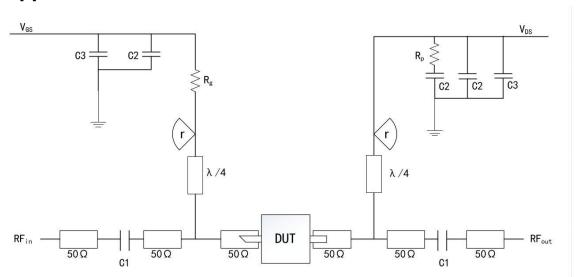
DUT: Device to be tested
