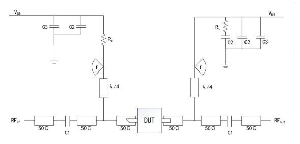
DUT: Device to be tested
