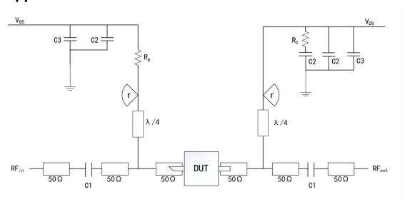
DUT: Device to be tested
