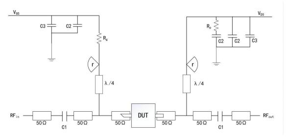
DUT: Device to be tested
