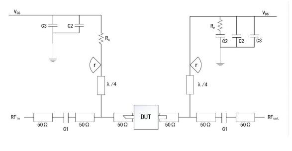
DUT: Device to be tested
