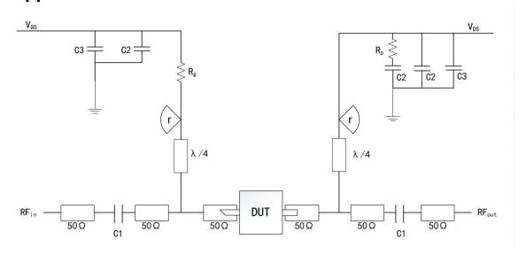
DUT: Device to be tested
