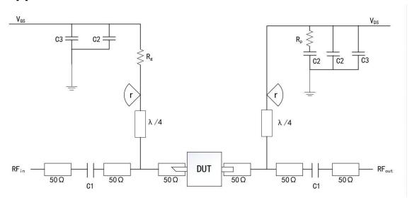
DUT: Device to be tested
