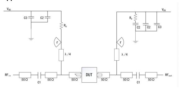
DUT: Device to be tested
