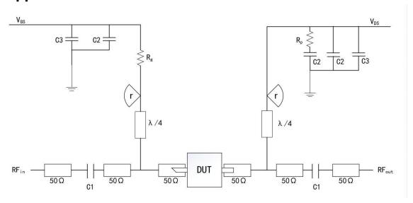
DUT: Device to be tested
