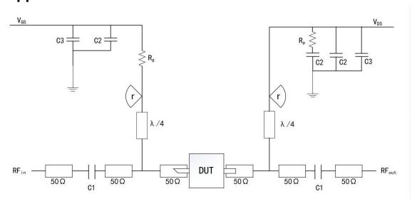
DUT: Device to be tested
