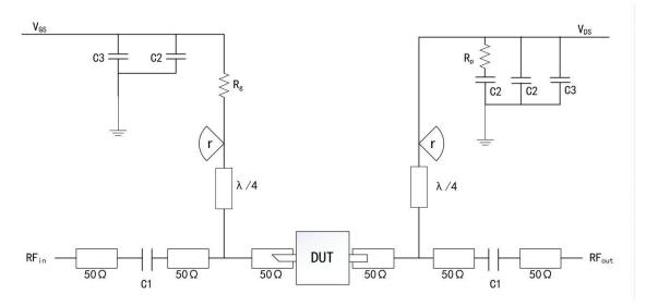
DUT: Device to be tested
